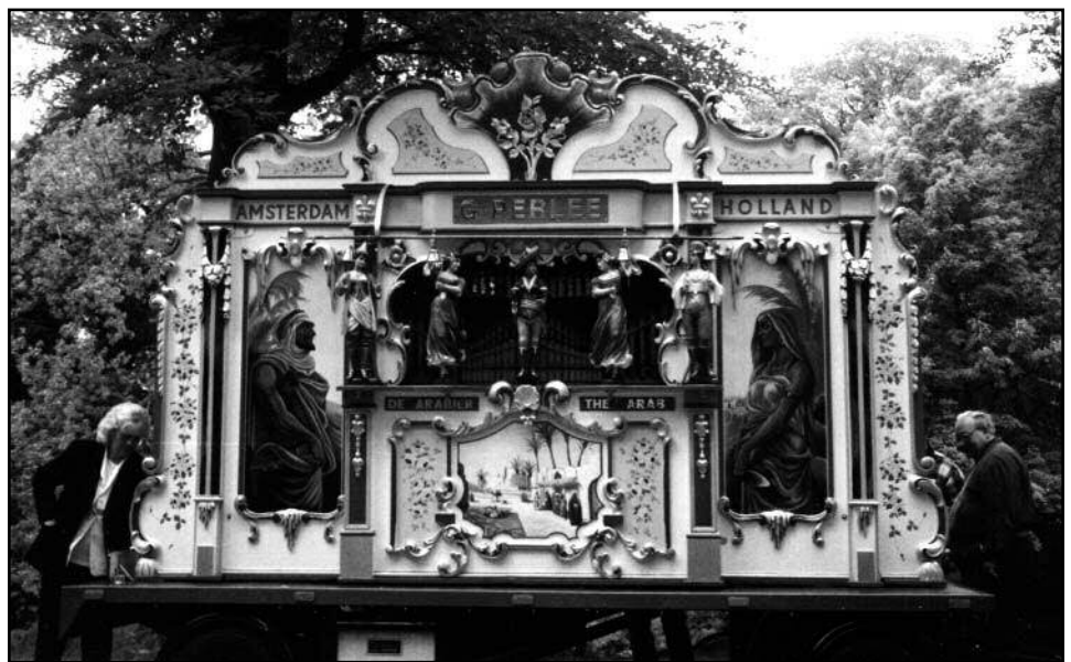
Figure 1. De Arabier —the most famous street organ in the Netherlands. It was built by P. Verbeeck in Belgium in the 1920s. It was delivered without statues and without trombone pipes. In 1948 the organ was rebuilt by Gijs Perlee in Amsterdam, who changed some registers and built in the classical bourdon céleste. From the 1950s more and more statues were added to the organ—first three, then five and then, seven! In the early 1960s it had no less than nine statues. By then the organ was slightly spoken of as de Poppenkast (the Punch and Judy show). Today the amount of statues have been reduced to five—five more than when the organ was shipped.
